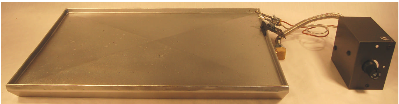
FIGURE 20 – FIRE ISLAND BURNER PAN WITH VALVE – FRONT VIEW
